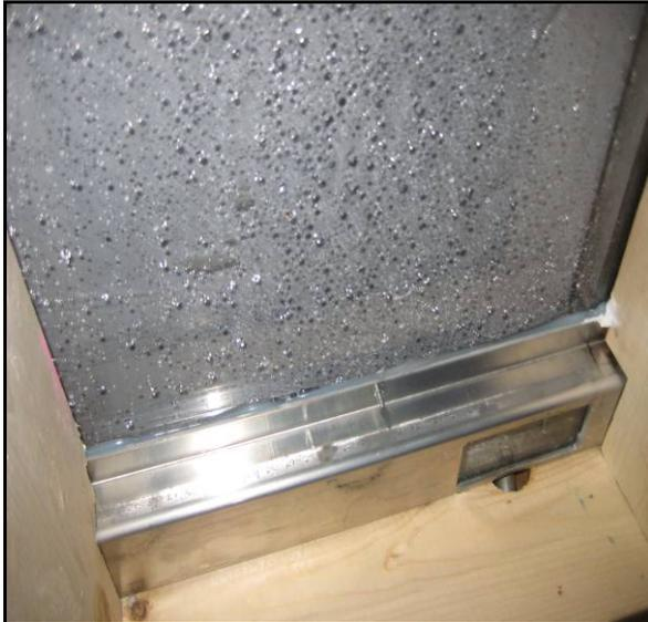
**Figure 4: Gutter Behind Cladding System at Sill of Drained and Back Ventilated Rain Screen Wall Cladding System (Allows for Collection of Water on Face of AWB)**
